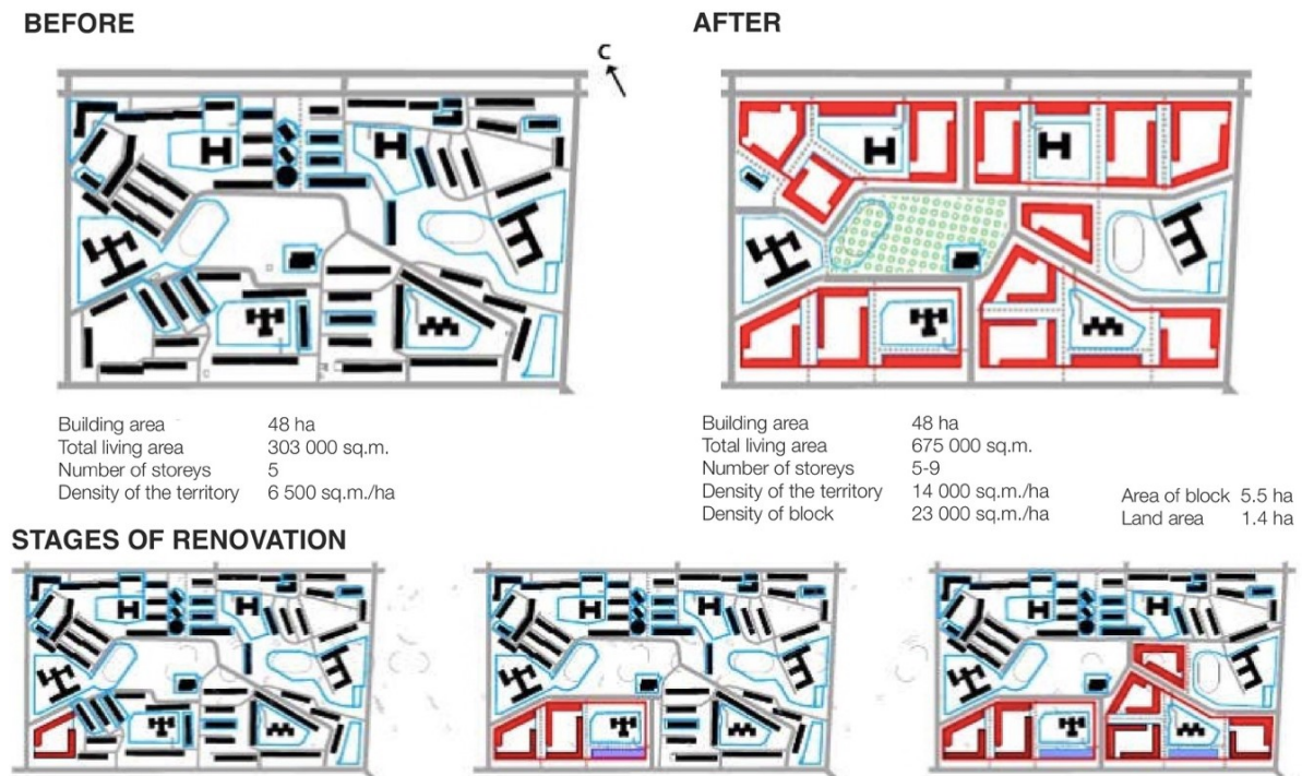
Figure 4. Project of renovation of microdistrict №2 with demolition of existing panel houses. Source: architectural buro "Ostozhenka"
