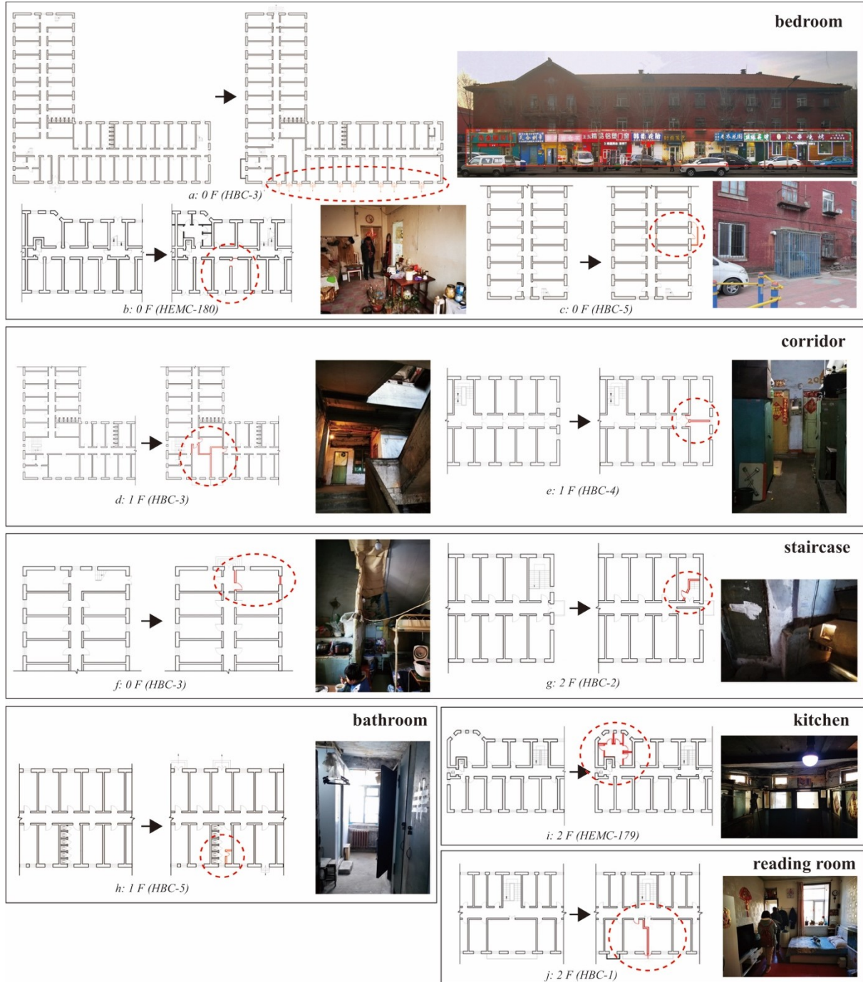
Figure 2. Informal transformations in Soviet-style housings, VoP (Source: Yiping Zhang)
